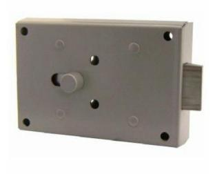
Surface mounted slam latch for FB4 Fire Brigade key Case size 110mm 78mm x 20mm Backset 54mm 4 way reversible - suitable for left or right handed doors, opening in or out Supplied with 2 x strike plates (1 x flat and 1 x surface mounted), 1 x escutcheon and all fixing screws FB4 Slam latch - FB4M
